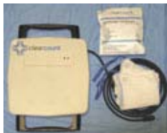
The Clear Count RFID system includes a reader wand to identify the sponges.
