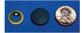
Each RFID tag is the size of a penny and contains no batteries.
