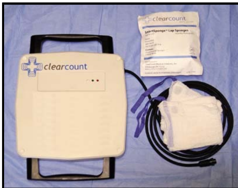
“Wand” device (left) and special sponges embedded with RFID tags. Courtesy of ClearCount.
