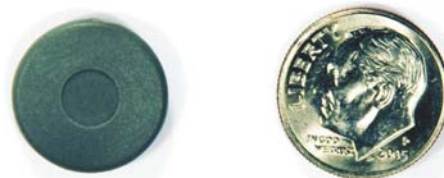
Dime-sized SmartSponge tags can be detected quickly and accurately through blood and bloody tissue.
